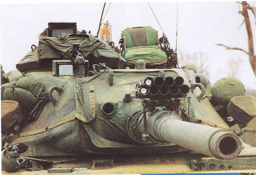
(Left) The nine-tube muzzle blast simulator and the way it is mounted on the main gun barrel. Covers are installed over the smoke dischargers. The fake laser range finder can be seen on the left side of the turret.
