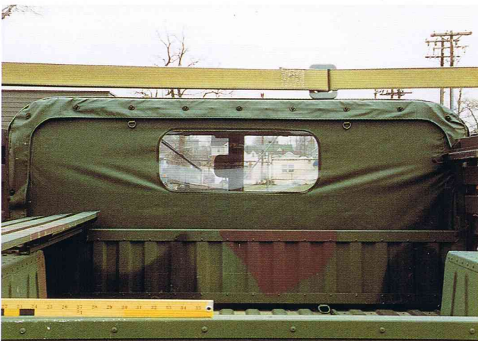
To prevent stowage from entering the front cabin, a bulkhead was installed just aft of the driver's seat. Note the rear view window in the soft skin top and the way the top cover slips over the rear cover. Attachment is by press-and-pull buttons.
