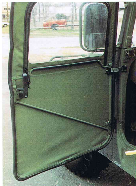
The inside of the soft skin door with the cross-bar for additional strength. Note the handhold and the door latch.
