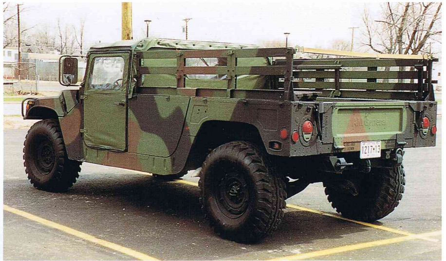
An overall view of the vehicle. The 16 inch (40cm) ground clearance and the large wheel base are apparent in this picture. Note the green, black and brown camouflage pattern is not applied to the soft cover. Also note the sling on the rear of the bay and the black and white US Army license plate.
