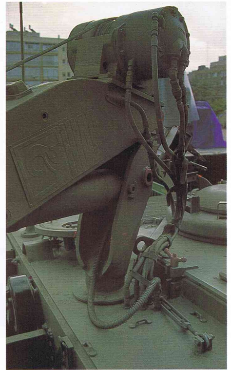
All of the hoisting crane's hydraulic lines protrude from the upper deck on the left side of the crane.
