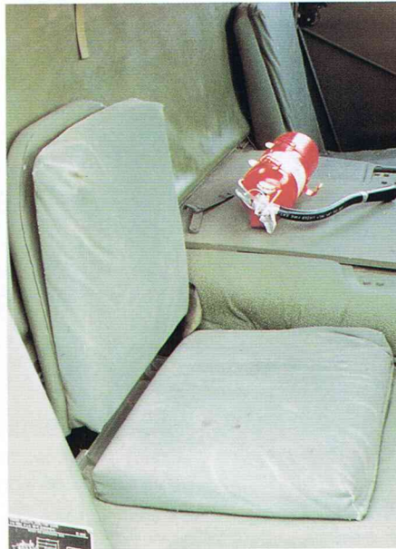
A view on the area in-between the two seats in the front cabin, featuring a fire extinguisher within reach of each crewmember.
