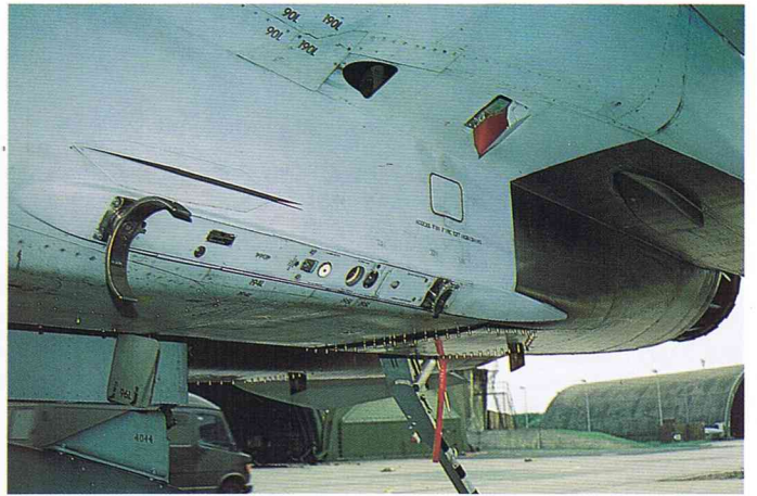
Fig.11 One of the aft Sparrow launch rails on the bottom of the fuselage. The kit is lacking all the detail, but this can be changed using VP's update set.
