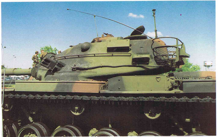
The top loading air cleaner on top of the left fender, the additional cheek fillets on both sides of the gun mantlet and the thick armored skirts on the bottom of the turret are M60A3 characteristics.
