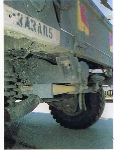
This look on the mattock storage area shows the way the cargo compartment is attached to the chassis by means of shock-absorbing rubber pads.
