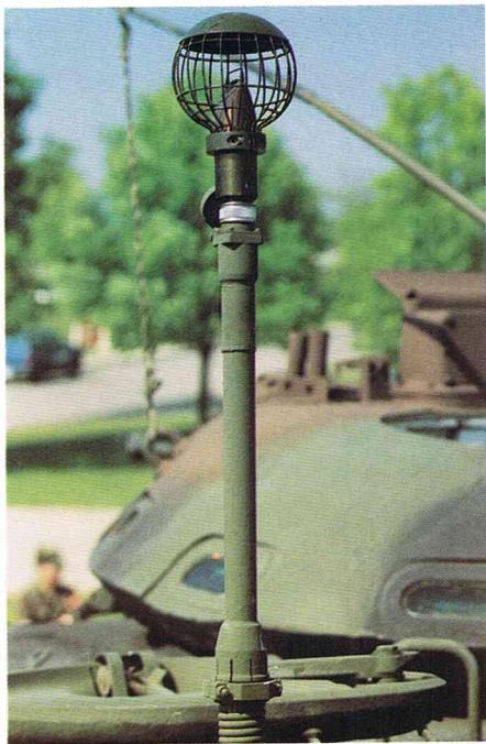
The crosswind sensor on top of the M60A3 turret, seldom shown in such detail. Kit parts can be updated accordingly.
