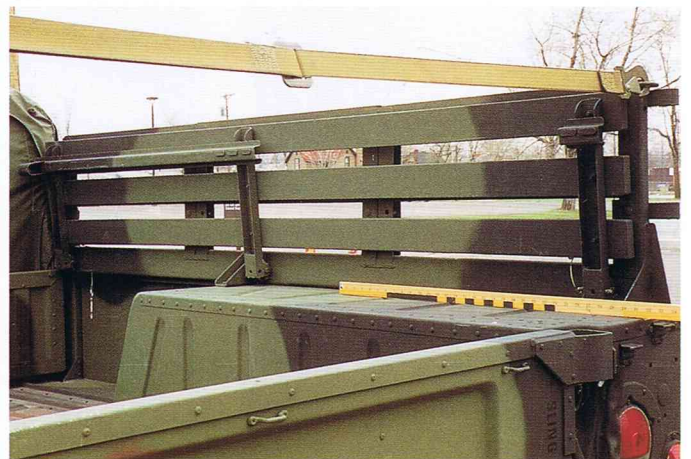
Raising the troop carrier's seat reveals the support bar attached to it which spans the gap over the rear passenger's seat location.
