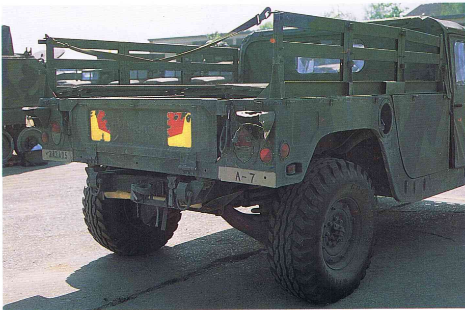
A shovel and a mattock are stowed just aft of the rear wheelbase and underneath the cargo bay. Note the various markings on this 3rd Armor Division Humvee.
